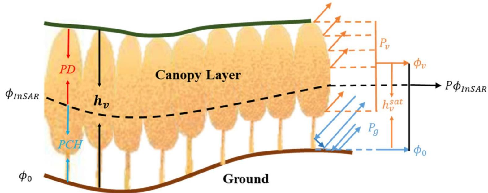
The saffron color denotes the volume scattering from the canopy layer, with phase center  $\phi_v$ . The blue color represents the ground scattering, with phase center  $\phi_0$ . The InSAR backscattered signal consists of the superposition of both; hence, with phase center  $\phi_{InSAR}$ .
