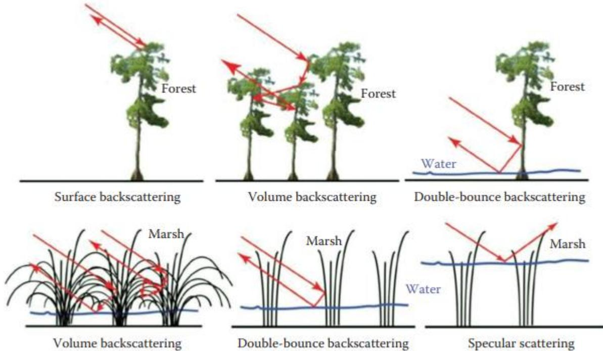
Schematic illustrating the different microwave scattering processes for forest and wetland vegetation (Brisco, 2015)
