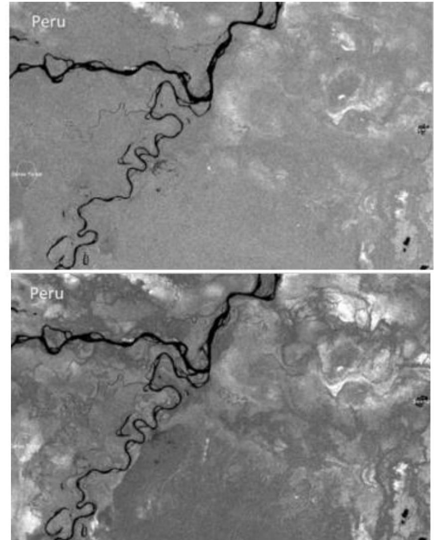
Double-bounce effect from bellow-canopy flooding at L-HH polarization from ALOS-1:
