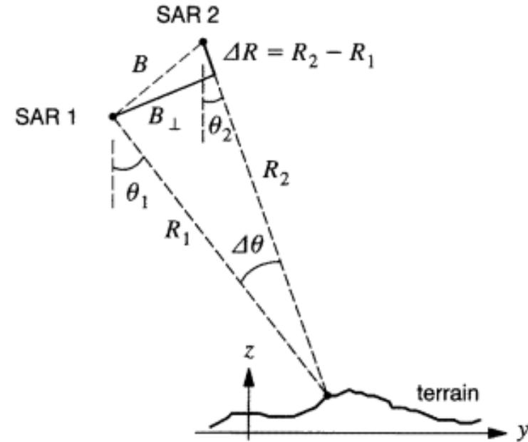
Across-track SAR interferometer (flight paths perpendicular into plane).
